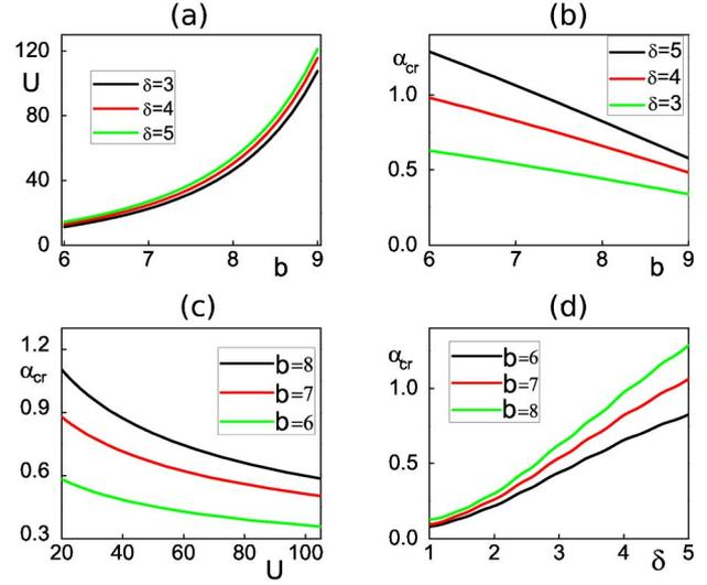
Fig. 2. Properties of ground-state solitons in quasi-one-dimensional lattices with single channel. (a) Energy flow versus propagation constant. (b) Critical tilt versus propagation constant. (c) Critical tilt of the solitons versus energy flow. (d) Critical tilt versus modulation parameter. In all cases,  $k_t = 20$ .
