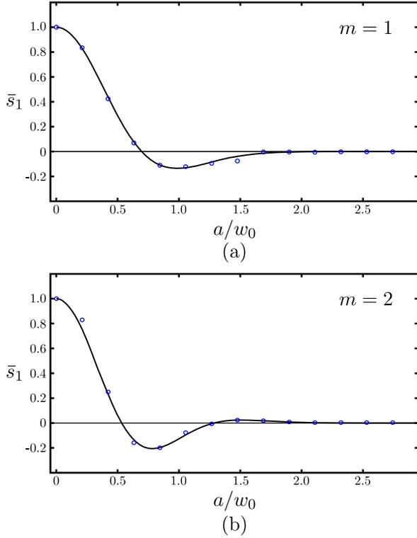
Fig. 3. Global normalized Stokes parameter  $\bar{s}_1 = \bar{S}_1/\bar{S}_0$  as a function of the normalized separation  $a/w_0$  for a diagonally polarized LG beam with azimuthal orders (a)  $m = 1$  and (b)  $m = 2$ , theoretical (solid line) and experimental (circles).
