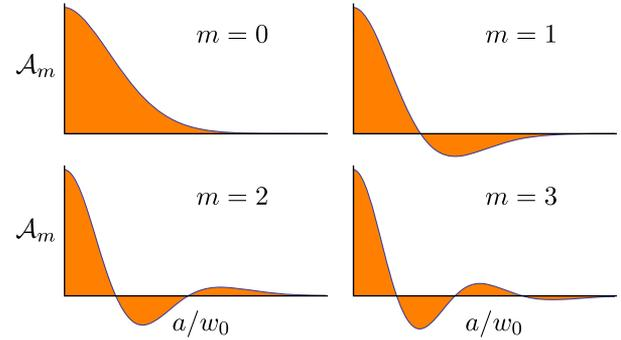
Fig. 1. Autocorrelation function of a LG beam for different azimuthal orders  $m$ .
