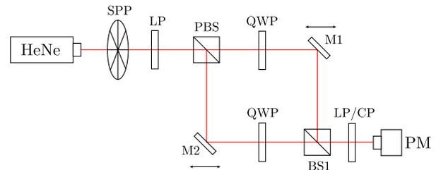
Fig. 2. Experimental setup to observe the autocorrelation function  $\mathcal{A}_m(a, 0)$ .
