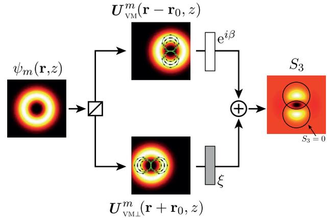
**Figure 1.** Schematic representation of the off-axis superposition of orthogonal doughnut vector modes to find the topological charge  $m$ .
