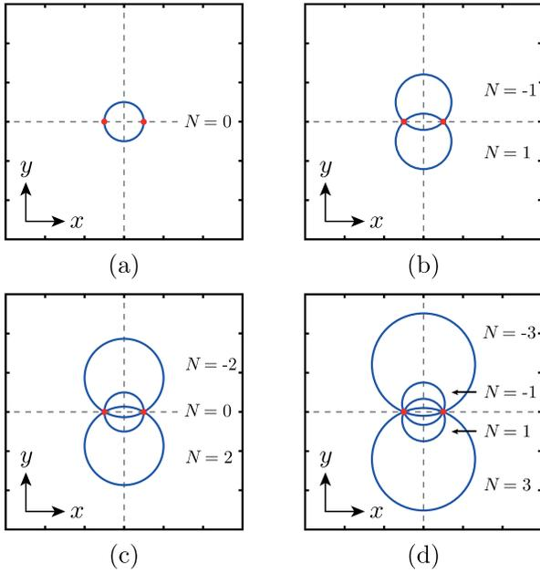
**Figure 2.** Solutions of  $S_3 = 0$  for a superposition of orthogonal vector modes with a horizontal displacement of  $x_0 = 1/2$  for topological charges (a)  $m = 1$ , (b)  $m = 2$ , (c)  $m = 3$ , and (d)  $m = 4$ .
