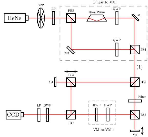
**Figure 3.** Experimental setup to generate the off-axis superposition of orthogonal vector modes.
