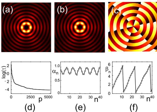
Fig. 1. (Color online) (a) Objective intensity pattern of a third order modulated Bessel beam and (b) intensity pattern obtained, using the genetic algorithm and (c) its phase distribution. All profiles are shown in a  $xy$  box of  $12 \times 12$  with  $k_t = 4$ . (d) Evolution of the error function. (e) Amplitude and (f) phase angular spectrum obtained with the genetic algorithm.
