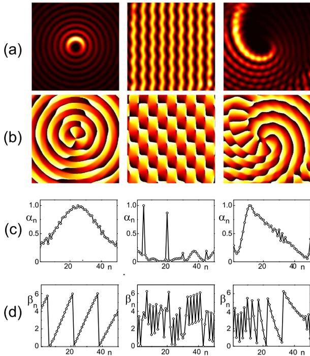
Fig. 3. (Color online) (a) Intensity, (b) phase, and (c) amplitude and (d) phase angular spectrum of unusual NBs that corresponds to an asymmetric Bessel beam, a zigzag cosine like beam and a spiral nondiffracting beam. All profiles are shown in a  $xy$  box of  $12 \times 12$  with  $k_t = 3$  for the zigzag case, and  $k_t = 4$  for the rest.
