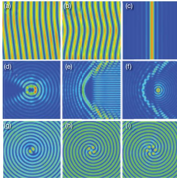
Intensity distributions in quasi-nondiffracting beams constructed via angular spectrum engineering. Top row shows bent (a), curved (b), and stripe-like (c) beams. Middle row shows truncated Mathieu (d), parabolic-cosine (e), and parabolic-Bessel (f) beams. Bottom row (g)-(i) shows specific spiraling patterns.
