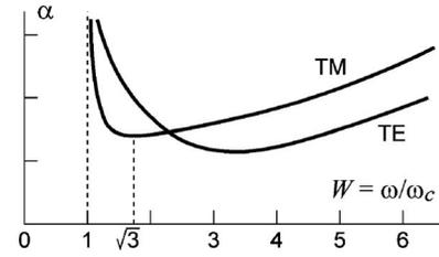
Fig. 3. General behavior of the attenuation constants as a function of the normalized frequency  $W$  for both TM and TE modes.
