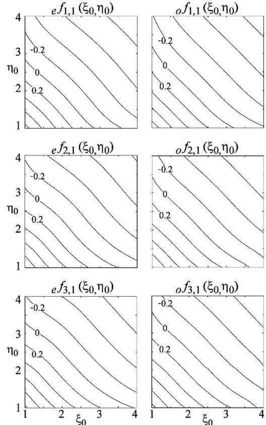
Fig. 4. Contour plots of  $\log(f_{m,n})$  on the plane  $(\xi_0, \eta_0)$  for the lowest order even and odd modes. Labels corresponding to  $\log(f_{m,n}) = \{-0.2, 0, 0.2\}$  are included in the plots; remaining labels have been omitted for clarity. For all plots, the separation between consecutive contour lines is 0.2, and  $1 \leq \xi_0 \leq 4$  and  $1 \leq \eta_0 \leq 4$ .
