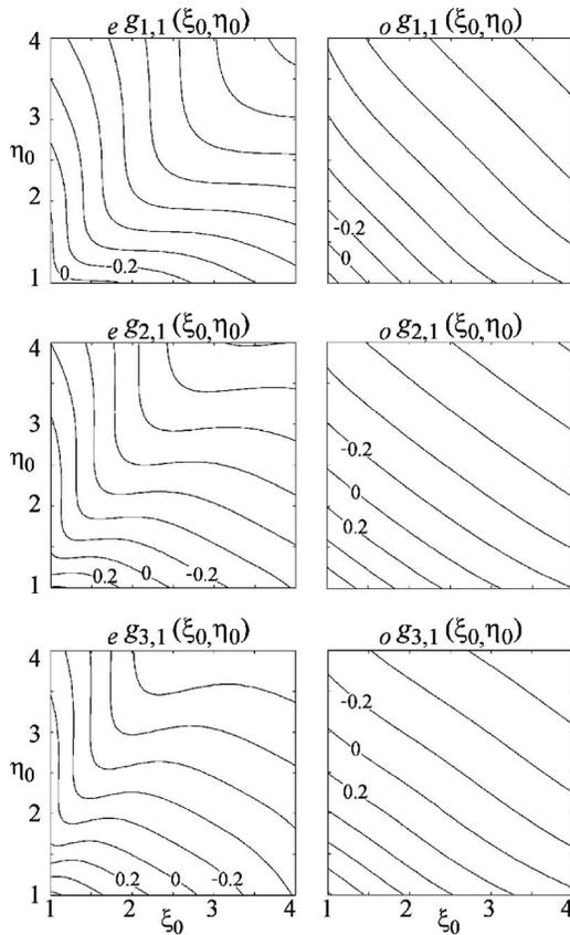
Fig. 5. Contour plots of  $\log(g_{m,n})$  on the plane  $(\xi_0, \eta_0)$  for the lowest order even and odd modes. Labels corresponding to  $\log(g_{m,n}) = \{-0.2, 0, 0.2\}$  are included in the plots; remaining labels have been omitted for clarity. For all plots, the separation between consecutive contour lines is 0.2, and  $1 \leq \xi_0 \leq 4$  and  $1 \leq \eta_0 \leq 4$ .
