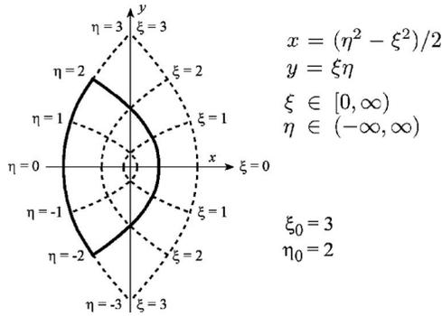
Fig. 1. Geometry of the parabolic waveguide and the definition of the parabolic coordinates.
