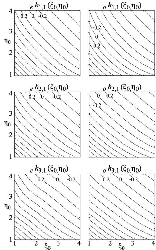
Fig. 6. Contour plots of  $\log(h_{m,n})$  on the plane  $(\xi_0, \eta_0)$  for the lowest order even and odd modes. Labels corresponding to  $\log(h_{m,n}) = \{-0.2, 0, 0.2\}$  are included in the plots; remaining labels have been omitted for clarity. For all plots, the separation between consecutive contour lines is 0.2, and  $1 \leq \xi_0 \leq 4$  and  $1 \leq \eta_0 \leq 4$ .
