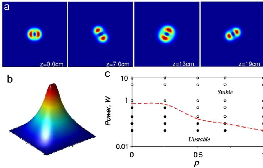
Fig. 3. (a) Example of a stable rotating dipole soliton in a thermal nonlocal nonlinear medium; (b) the spatial profile of the refractive index change induced by a dipole soliton with the contrast parameter  $p = 0.7$  and input power 5 W; width of the computational window is  $200\ \mu\text{m} \times 200\ \mu\text{m}$ ; and (c) stability domain for the rotating dipole solitons for the parameters  $(p, P)$ .
