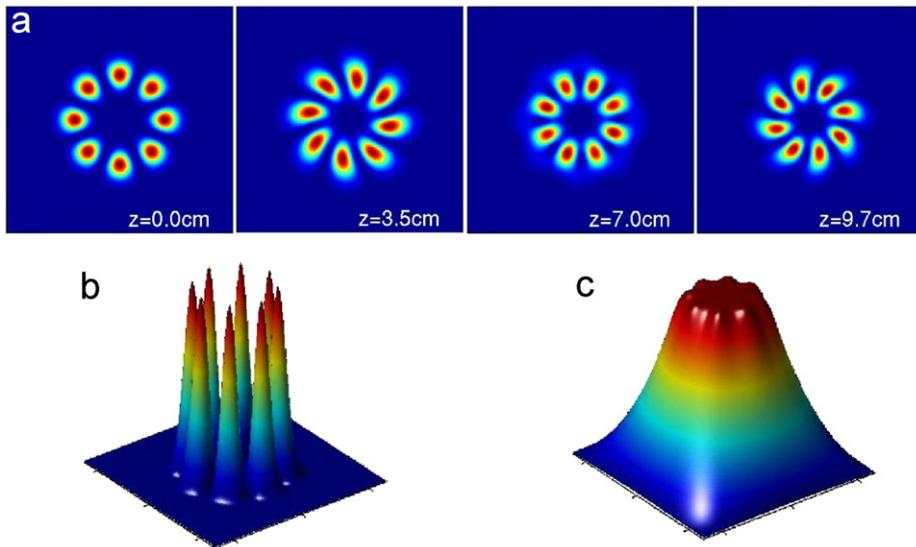
Fig. 4. (a) Example of a stable rotating necklace soliton in a thermal nonlocal medium; input power 5 W; width of the computational window  $200\ \mu\text{m} \times 200\ \mu\text{m}$ . (b,c) Surface plots of the intensity and refractive index profile, respectively.
