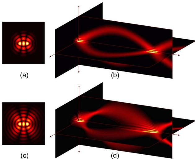
Fig. 1. (Color online) Propagation of an ordinary  $MG_2(\mathbf{r}, \varepsilon=8)$  beam through a GRIN medium from  $p=0$  to  $p=2.5$ . (a), (b) Constant Gaussian width. (c), (d) Variable Gaussian width.
