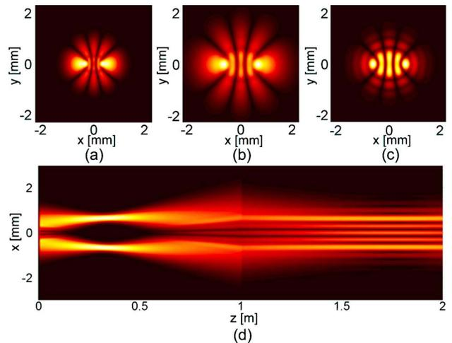
Fig. 2. (Color online) Propagation of a  $MG_4(\mathbf{r}, \varepsilon=8)$  ( $\kappa_1=-18394+i4751$  m<sup>-1</sup>,  $q_1=-0.331-i0.102$  m) through two free-space regions separated by a complex thin lens. Transverse field at (a)  $z=0$ , (b) after the complex lens  $z=1$  m, (c) at  $z=2$  m, (d) Evolution along the plane ( $z, x$ ).
