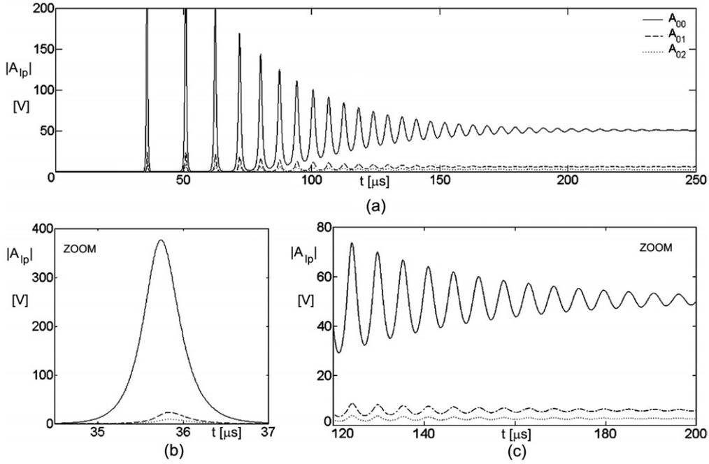
**Figure 5.** Temporal evolution of absolute value of the three lowest-loss modal amplitudes, using the seven lowest-loss  $l = 0$  transverse modes in the basis set. (a) Full evolution to a steady state. (b) Zoom of modal competition in the first laser spike. (c) Zoom of modal competition in relaxation oscillations.
