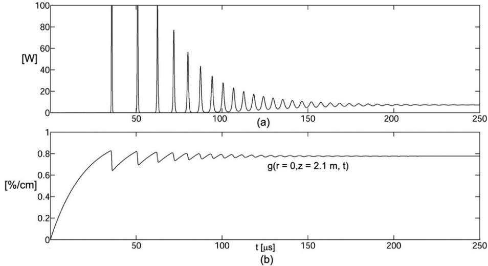
**Figure 6.** (a) Temporal evolution of computed laser output power without transverse hole burning. Behaviour depicts spiking and relaxation oscillations that evolve to a final steady state value. (b) Local gain [ $g(r = 0, z = 2.1 \text{ m}, t)$ ] build-up at a particular axial position; gain is partially depleted during the laser spike and evolves asymptotically to its steady state value.
