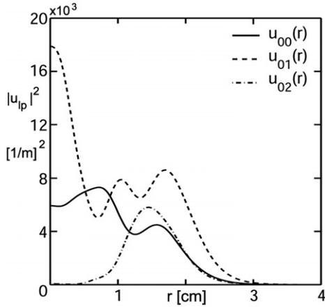
**Figure 2.** Transverse intensity distribution incident on the output mirror of the first three lowest-loss  $l = 0$  bare cavity eigenmodes.
