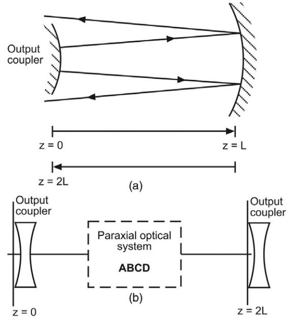
**Figure 1.** (a) Standing wave unstable resonator cavity. (b) Resonator lens equivalent system with single diffractive aperture. The reference plane is located just before incidence with the output coupler.
