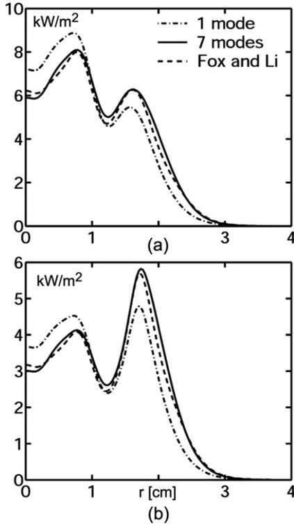
**Figure 4.** Steady state gain loaded (a) intracavity (incident on the output coupler) and (b) output intensity distribution. Results from the DCM method using one and seven transverse modes in the basis set are compared to those obtained from the iterative Fox and Li approach.
