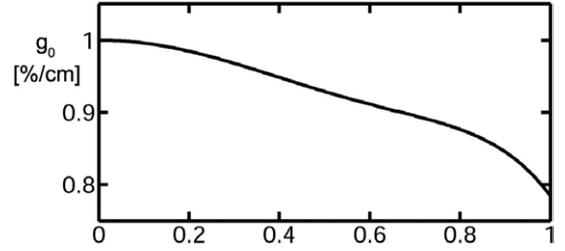
**Figure 3.** Radial variation of the implemented small-signal gain; the radial coordinate is normalized to the tube radius.
