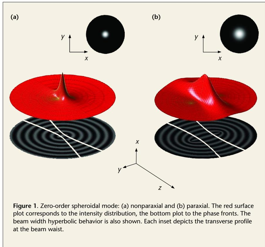
**Figure 1.** Zero-order spheroidal mode: (a) nonparaxial and (b) paraxial. The red surface plot corresponds to the intensity distribution, the bottom plot to the phase fronts. The beam width hyperbolic behavior is also shown. Each inset depicts the transverse profile at the beam waist.
