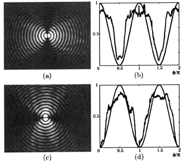
Fig. 4. (a) and (c) Photographic images of the first-order Bessel cosine and Bessel sine beams and (b) and (d) intensity variation with angular position for the fourth lobes.
