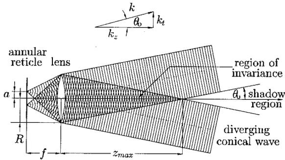
Fig. 1. Simple experimental setup used to generate nondiffracting beams.
