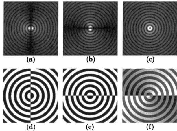
Fig. 2. Amplitude and phase distributions of the first-order (a) and (d) Bessel cosine, (b) and (e) Bessel sine, and (c) and (f) Bessel beams. In the phase distributions, white regions represent a value of zero and black regions represent a value of  $\pi$ .
