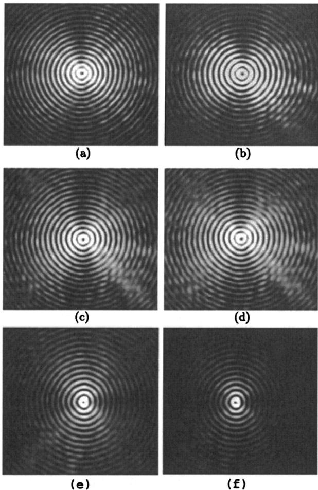
Fig. 5. Photographic sequence of the first-order Bessel beam at planes  $z = 1, 2, 3, 4, 5,$  and  $6$  m. Image size is  $1.8 \text{ mm} \times 1.8 \text{ mm}$ .
