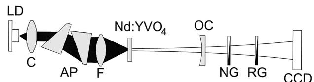
Fig. 1. Experimental arrangement for the observation of IGMs in a laser cavity: LD,  $\lambda = 808$  nm pump laser diode; C, collimating lens; AP, anamorphic prism pair; F, focusing lens; Nd:YVO<sub>4</sub>, laser crystal; OC, 97% output coupler; NG, neutral glass filter; RG, colored glass filter; CCD, camera.
