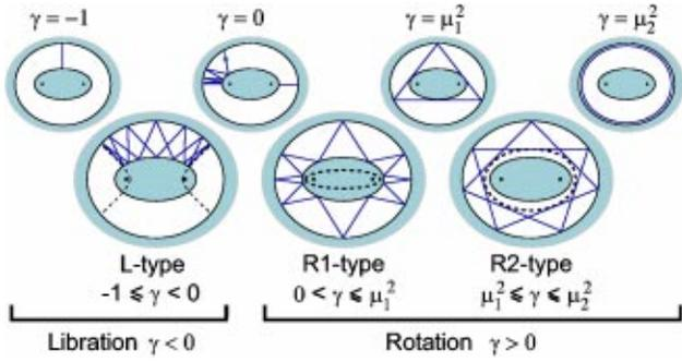
Fig. 2. Classification of the orbits in the confocal elliptic billiard. The dashed lines represent the caustics of the tori.
