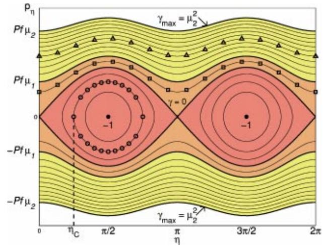
Fig. 3. Poincaré mapping  $(\eta, p_\eta)$  for the confocal elliptic billiard. The form of the lines is given by  $\gamma = \text{constant} = (p_\eta/Pf)^2 - \sin^2 \eta$ . Specific orbits are represented by circle markers for L motion, square markers for R1 motion, and triangle markers for R2 motion.
