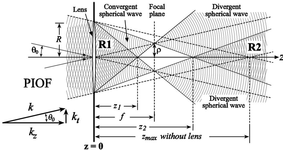
Figure 1. Geometrical evolution of the focusing of a PIOF.
