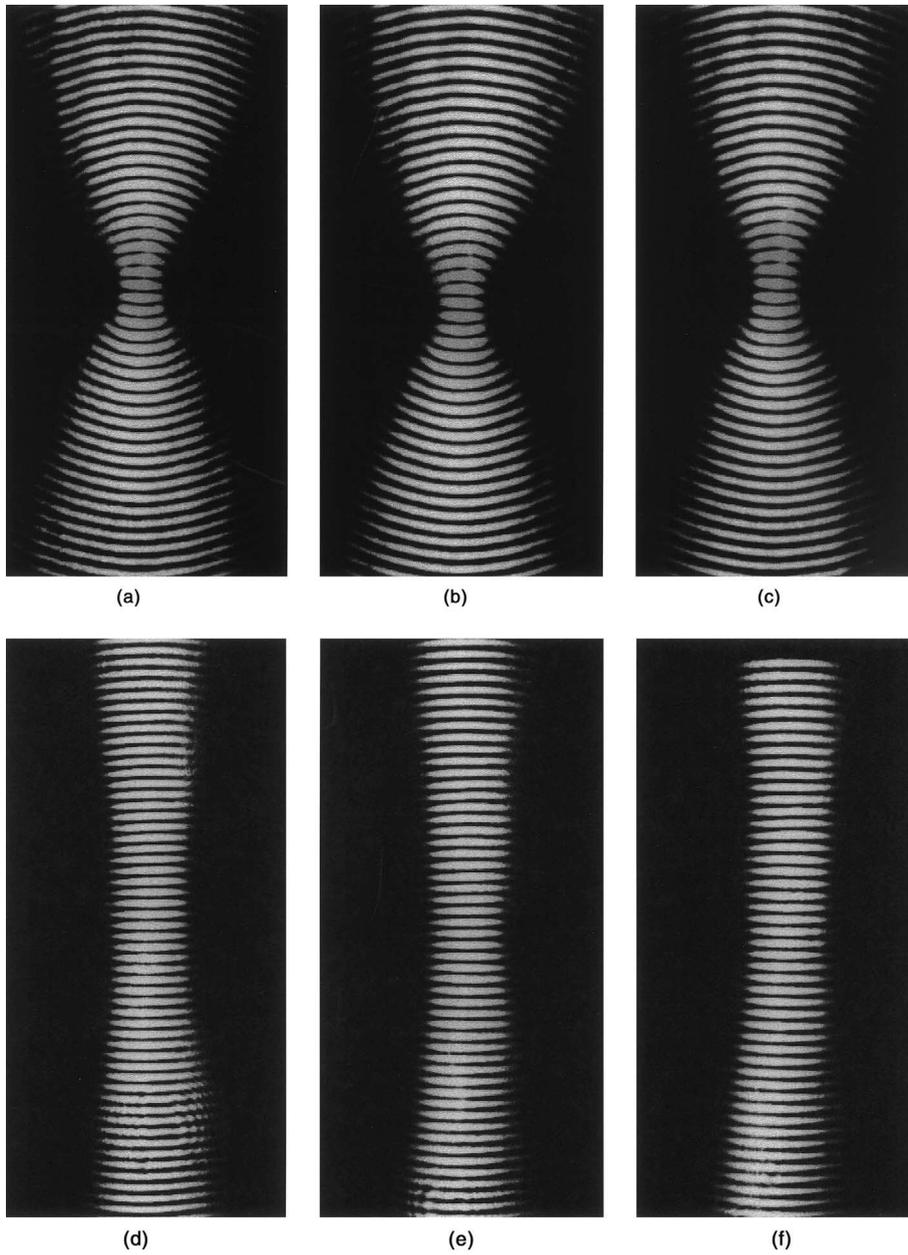
Fig. 4. Photographic sequence of transverse intensity patterns of zero-order Mathieu beams obtained experimentally at  $z = 0, 1$  and  $2$  m for (a–c)  $q = 25$ , and (d–f)  $q = 595$ .
