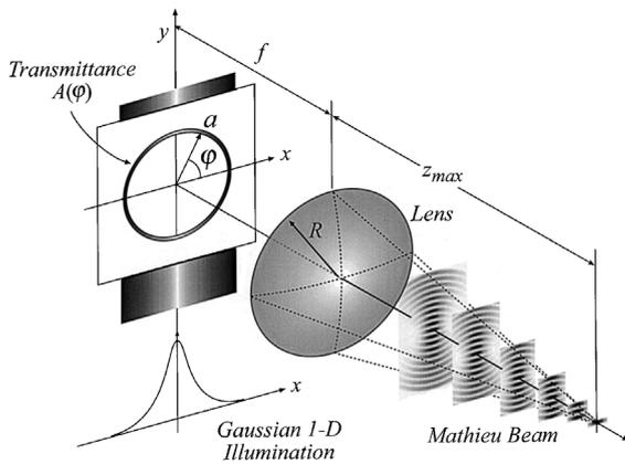
Fig. 3. Experimental setup to generate the zero-order Mathieu beam.
