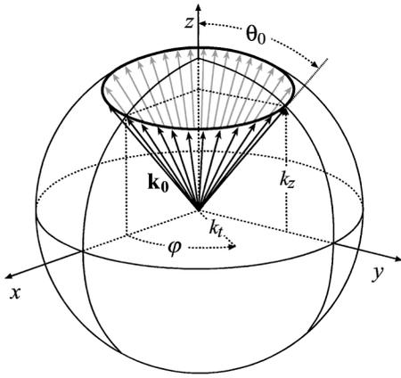
Fig. 1. IOF's are characterized by the ring formed by the intersection between the cone  $\theta = \theta_0$  and the McCutchen sphere  $|\mathbf{k}| = k_0$ .
