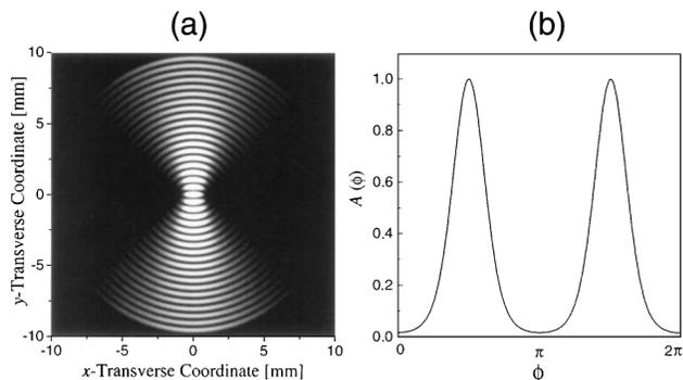
Fig. 2. (a) Transverse intensity pattern of a truncated zero-order Mathieu beam. (b) Angular spectrum of the zero-order Mathieu beam.
