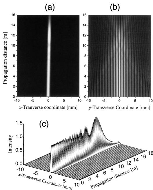
Fig. 3. Evolution of an apertured Mathieu beam on planes (a)  $x$ - $z$  and (b)  $y$ - $z$ . (c) Another view of the evolution in plane  $x$ - $z$ . One may observe the very well-defined quasi-invariant beam within the conic overlapping region.
